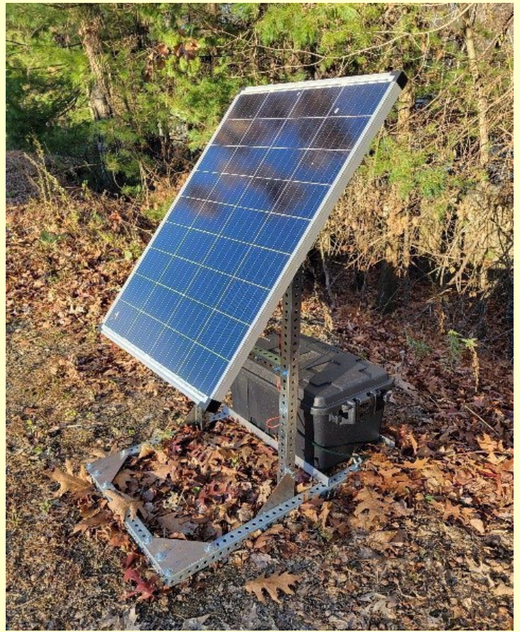
Image 6. Prototype to deliver solar power to our surveillance trap stations.
