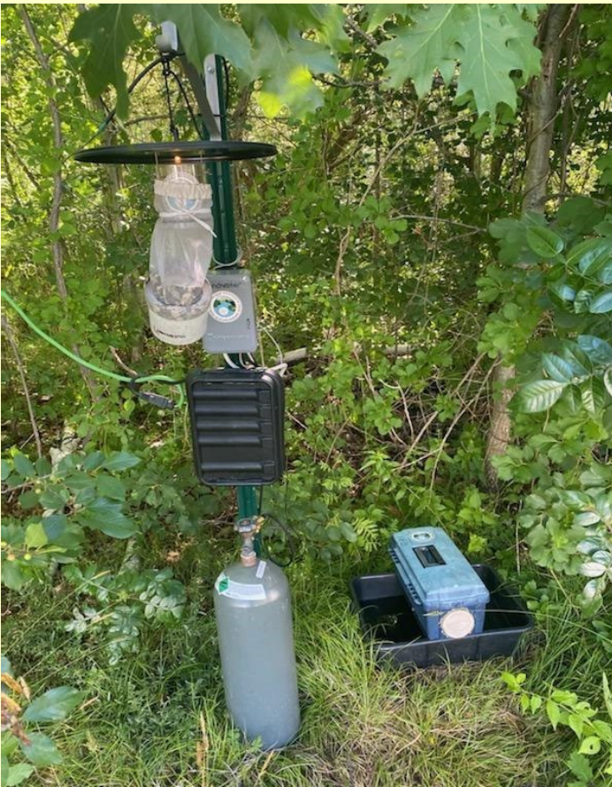
Image 5. Surveillance trap currently supplied by household electrical power.
