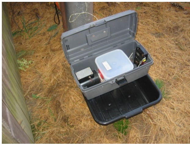
Figure 2. Reiter-Cummings Gravid Trap
